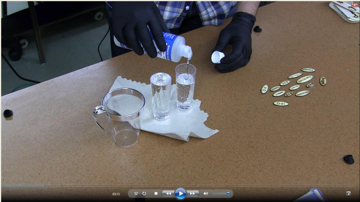
A two part clear cast epoxy resin was mixed in equal quantities and then poured over the mold.
