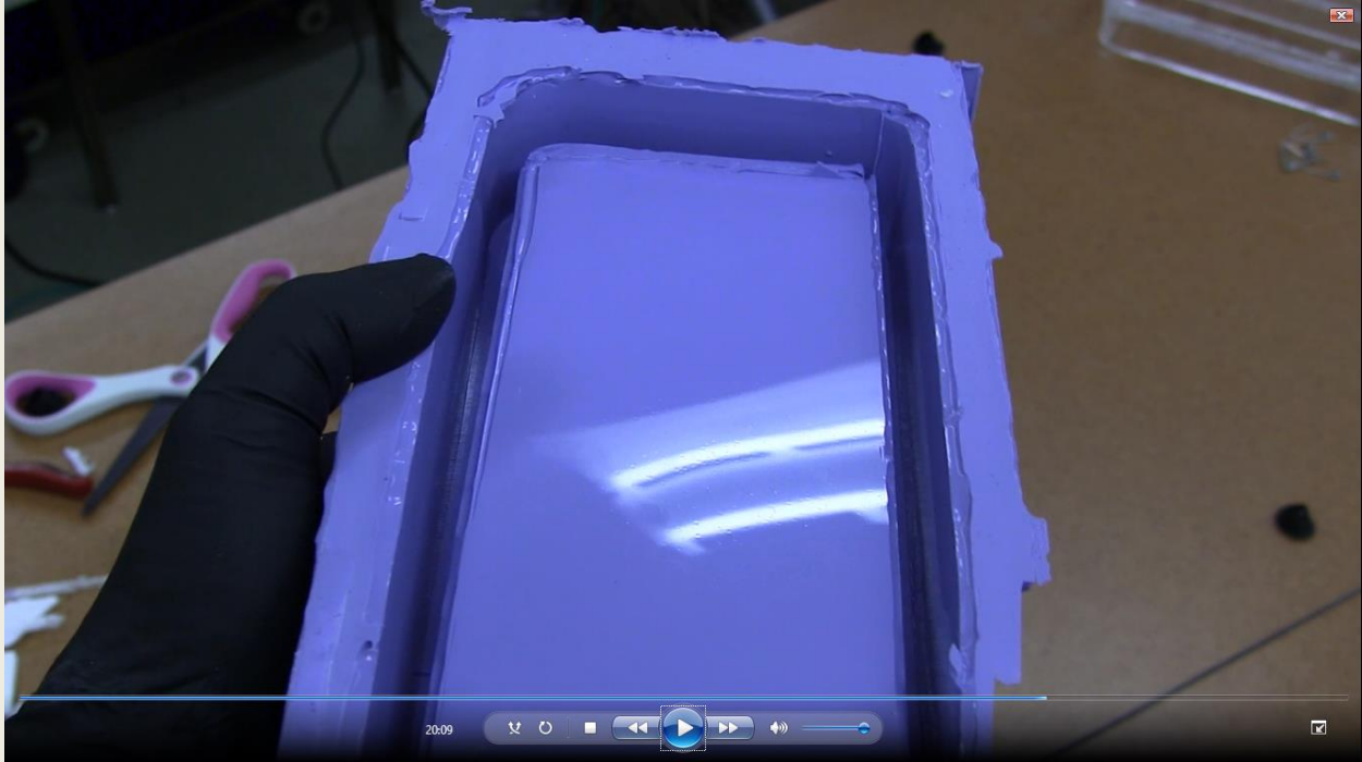
A two part clear cast epoxy resin was mixed in equal quantities and then poured over the mold.
